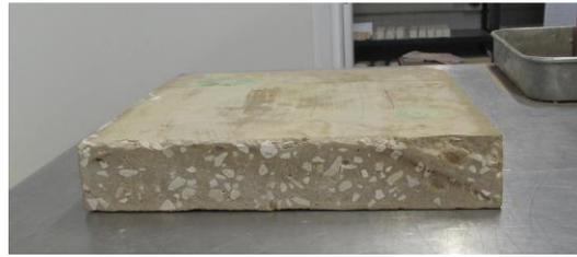
*Figure 3. Module composed sample type A 1:3:1 (cement; earth; gravel).*
