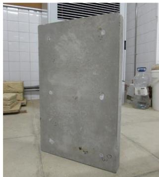
Figure 2. Standard concrete sample of the module.
