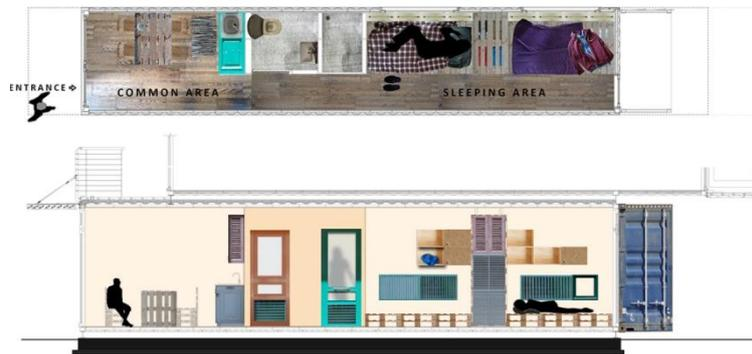
**Figure 6 Reuse of Materials: plan (above) and section (below) of the accommodation unit**
